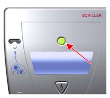
Fig. 2.1 Button to switch the device on and off, and to start the analysis (only in semi-automatic operation)
