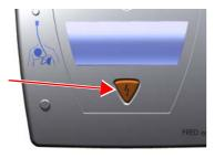
Fig. 4.8 Button to deliver the shock
