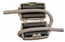
Fig. 5.6 Installing the cable within the ferrite core
